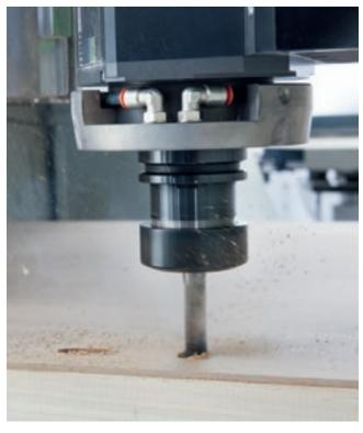
The Rover K Smart is equipped with 3 or 4 independent interpolating axes, and can be fitted with aggregates capable of handling any type of machining operation, both on panels and on solid wood workpieces.
