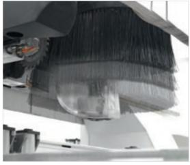
Suction cap adjustable on 6 positions allows a constant cleaning of the product and the surrounding area.
